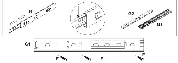
Need to assemble drawer runner in the correct pilot hole as the diagram indicates.
