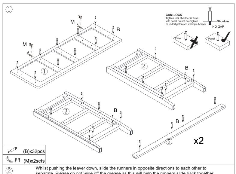
Whilst pushing the leaver down, slide the runners in opposite directions to each other to separate. Please do not wipe off the grease as this will help the runners slide back together at the end of assembly.
