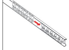
Hold the drawer horizontally and ensure the slide tracks are aligned to the runners. Push the drawer gently inwards until you hear a soft click.
