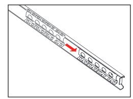
Hold the drawer horizontally and ensure the slide tracks are aligned to the runners. Push the drawer gently inwards until you hear a soft click.
